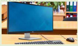
A monitor usually comprises the display device, circuitry, casing, and power supply. The display device in modern monitors is typically a thin film transistor liquid crystal display (TFT-LCD) or a flat panel LED display, while older monitors used a cathode ray tubes (CRT).
